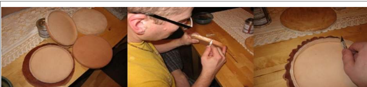
Illustration 2: Ends were made over a plywood last, lined, trimmed and sewn
