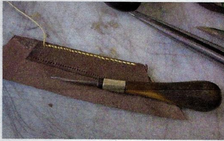
Line of Pricking from 7 to 14 per inch
